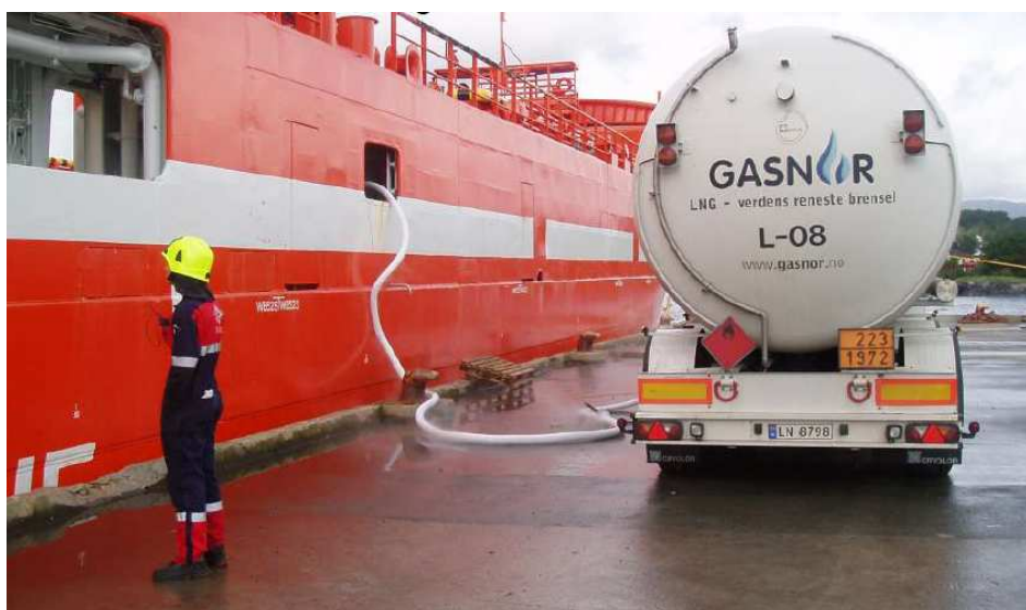
Figure 8. Bunkering of the vessel from tanker truck.
