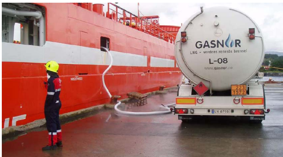
Figure 8. Bunkering of the vessel form tanker truck.
