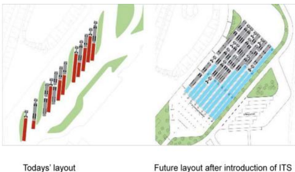
Figure 4 Arranging trucks in rows depending on departure Times utilizes more space (Source: EWTC)
