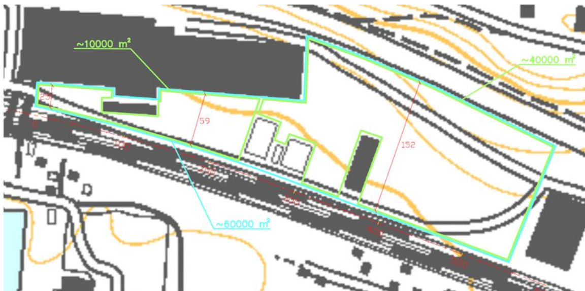
Figure 7. Example from Lahti: old industrial areas may offer facilities needed by first phase Dry Port. An essential issue is to find long enough rail and sufficient yard for the operations. Infrastructure must be very robust: weight of a reach stacker able to lift loaded containers is about 100 tons.
